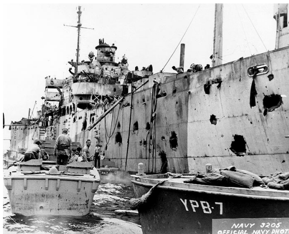
Port side of repair tender USS Mindinao (ARG 3), 350 yards from the explosion. Note the numerous holes; 82 of her crew were killed.
