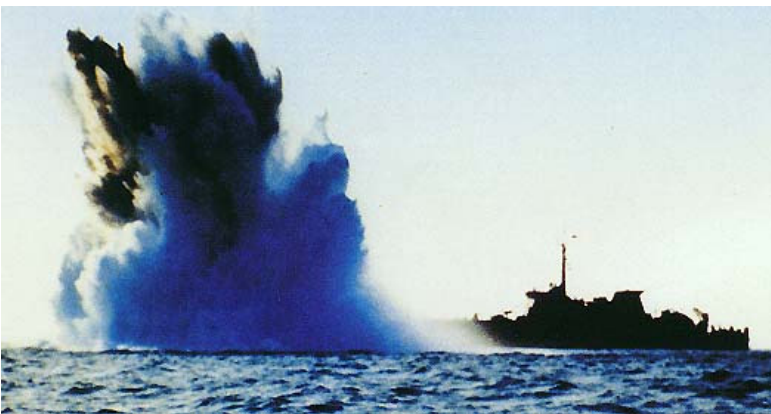
Minesweeper exploding a mine that had been swept to the surface, with gunfire from a stand-off distance. Note the size of the explosion versus the size of the ship.
